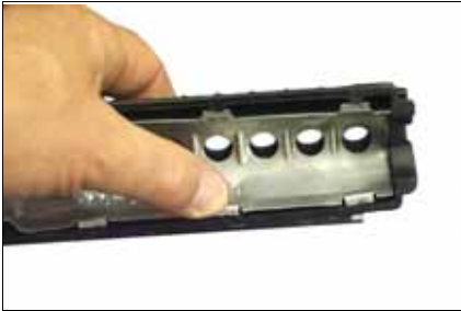
43. Gently re-install the heat shield.
